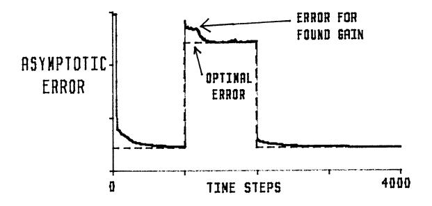
FIGURE C.2. Computer simulation of the single level adaptive gain selection algorithm. In this experiment the observation noise standard deviation parameter was step changed from sB=0.3 to sB=2.0 and then back again while the random movement standard deviation parameter remained constant at 1.0. These changes were made at the 1000th and 2000th time steps respectively.
