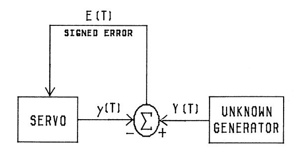
FIGURE C.1. A block diagram of a simple tracking servomechanism. y(t) is the pursuing function, Y(t) the target function, and E(t) the signed error.
