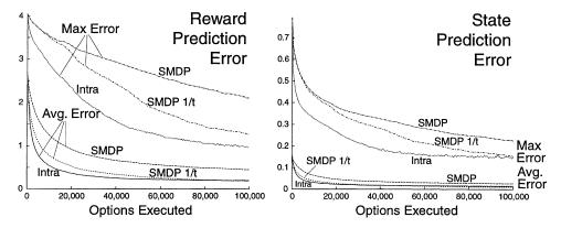
Fig. 9. Model learning by SMDP and intra-option methods. Shown are the average and maximum over  $\mathcal{I}$  of the absolute errors between the learned and true models, averaged over the eight hallway options and 30 repetitions of the whole experiment. The lines labeled 'SMDP 1/t' are for the SMDP method using sample averages; all the others used  $\alpha = 1/4$ .
