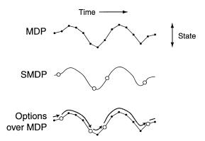
Fig. 1. The state trajectory of an MDP is made up of small, discrete-time transitions, whereas that of an SMDP comprises larger, continuous-time transitions. Options enable an MDP trajectory to be analyzed in either way.
