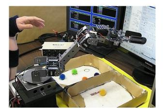
Figure 3: A table-top robot arm used to train new amputees. The multiple functions of the robot are selected and controlled using electrical recordings from three of the user's muscles, as processed by a real-time control computer.
