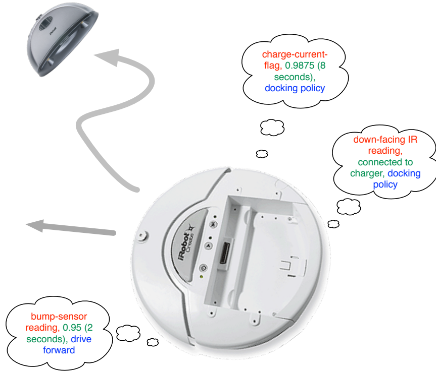
Figure 4.2: Several GVFs can be specified for a robot exploring it’s world. The red text specifies the cumulant signal, the green text specifies the termination signal, and the blue text specifies the target policy for each GVF. In this example, the behavior policy is random, selecting from a discrete set of actions with equal probability. We can specify several GVFs and approximate each in parallel from a single interaction stream produced by one robot.
